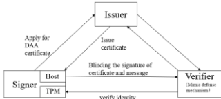
Fig. 2 Improved DAA protocol operation mechanism diagram
